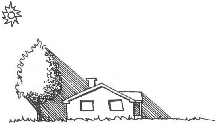
FIGURE 6.1. Direct solar radiation travels in straight parallel lines, casting predictable shadows.
